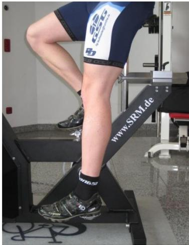
A person is standing on an SRM ergometer, adjusting the saddle height. The person's leg is extended downwards, and the heel of their shoe is touching the lowest point of the pedal. The ergometer frame has 'www.SRM.de' printed on it.                                            | <p><b>Saddle height</b></p> <p>The heel with the extended leg should reach the lowest position in the pedaling cycle.</p>                  |
