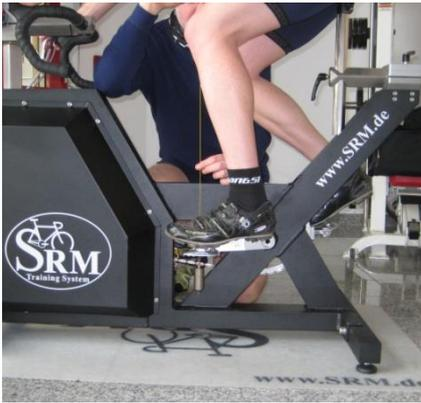
A person is sitting on the SRM ergometer, adjusting the saddle setback. The person's knee is positioned over the pedal in a horizontal crank position. The knee (patella) is perpendicular to the pedal axle. The ergometer frame has the SRM logo and 'www.SRM.de' printed on it. | <p><b>Saddle setback</b></p> <p>In the horizontal position of the crank the knee (patella) should be perpendicular to the pedals axle.</p> |
