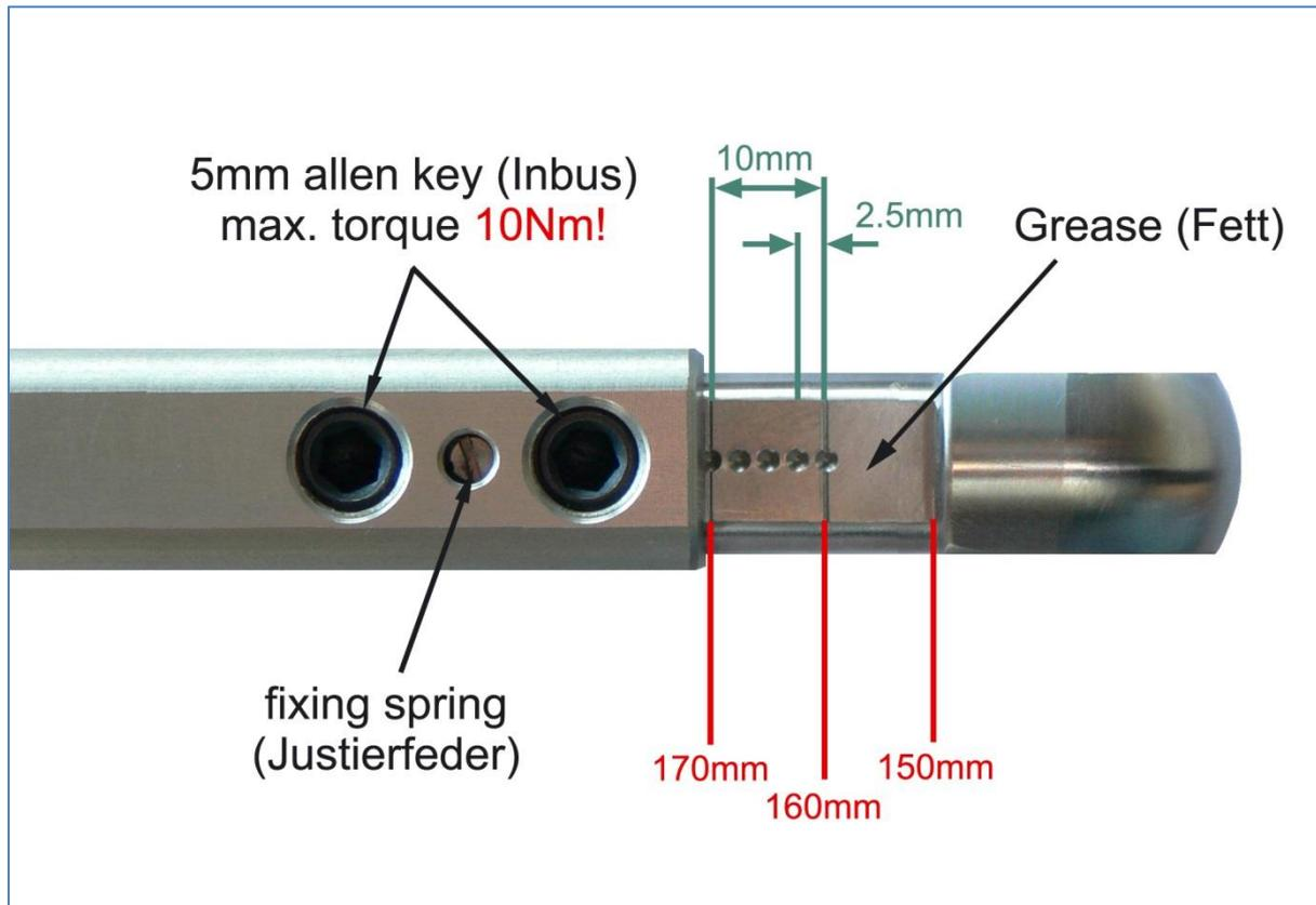
From time to time it is necessary to grease the steel elements of the crank to protect them from sweat and to maintain the free movement.
