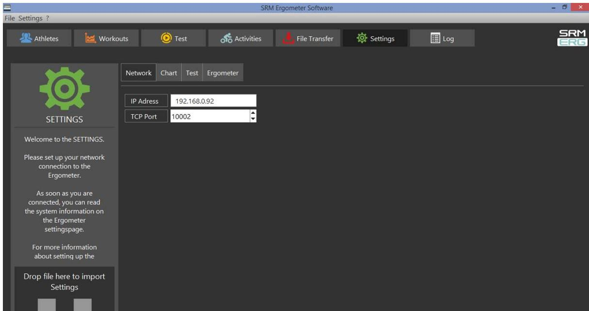
Choose a free and valid IP address (192.168.0.x) for your computer in the same sub network as the SRM Ethernet Torque Analysis Box (To install the Torque Analysis Box see the manual of the Torque Analysis).
