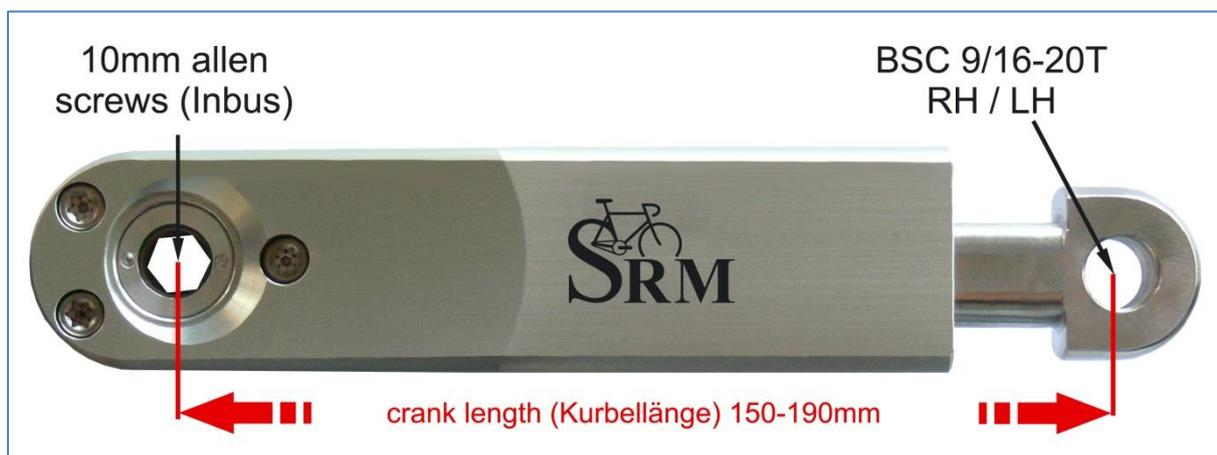
After adjusting the right crank arm length, please tighten the Allen screws again with a maximal torque of **10 Nm** so that they won't come loose while you ride the Ergometer. Make also sure that the screws are situated with a distance of a 2.5 mm. This can be determined when the fixing spring (situated between the Allen screws) locks into the holes of the steel element of the crank. Please do never remove or adjust the fixing spring.
